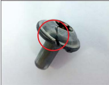
Typical cracked parts that were detected
