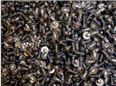
100% crack free parts waiting for the thread rolling operation.
