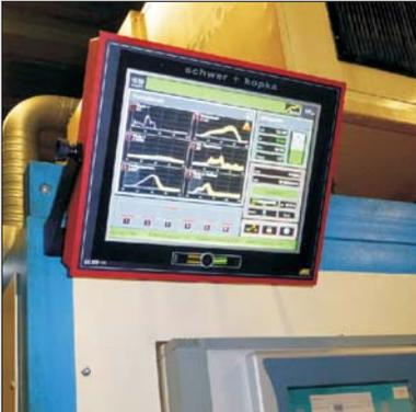
All multi die cold forming machines use the **SK 800** process monitoring terminal with its' large 15" touch screen.
