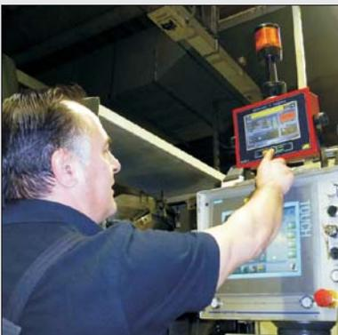
All thread rolling machines and a number of secondary machines are equipped with the compact monitoring terminal **SK 400** featuring a 7" touch screen.
