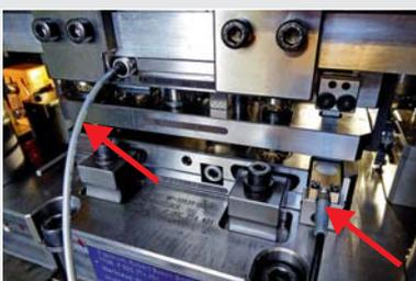
This tool uses both sensing systems in parallel: eddy current and force acoustic emission. The right cable comes from the eddy current sensor, the left one connects to the force and acoustic emission sensor mounted in the top stripper plate.
