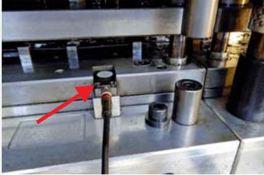
This figure shows a classic analog proximity sensor (eddy-current sensor) with its' sensor cable. Both sensor and cable are protected by the recessed installation. SK's state-of-the-art evaluation software significantly increases the monitoring results of the existing sensors as well.
