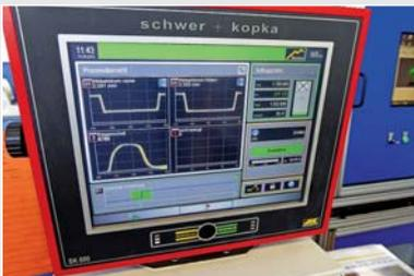
The monitoring system from SK monitors older proximity sensors and hybrid force-acoustic emission sensors in parallel. Thanks to modern monitoring software, the sensitivity of the proximity sensors has been improved as well. For old and new to interact, Schwer + Kopka has developed a unique sensor combination box.
