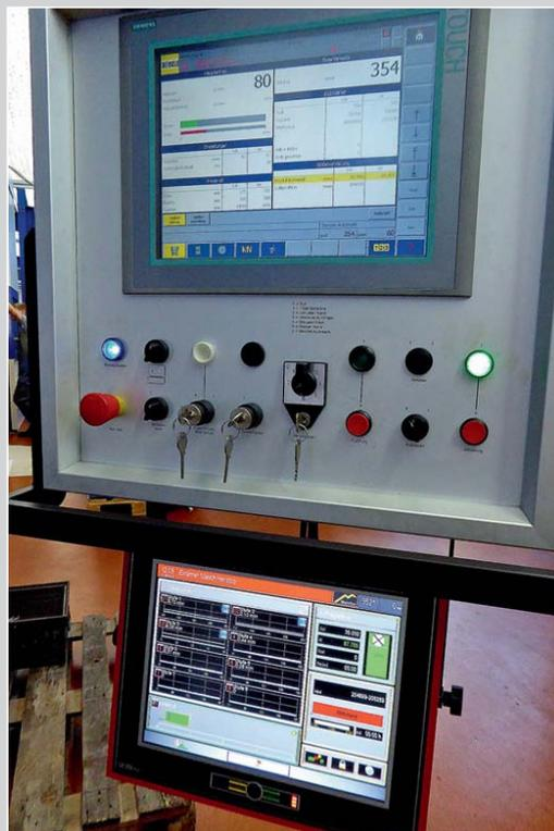
Left: in this case, the monitoring system by Schwer + Kopka is attached below the press control panel. The combination box with the eddy current and force-acoustic-emission-signal processing options helps ensure that the millions of very small precision stamped parts that are produced on the press are all of the highest possible quality.
