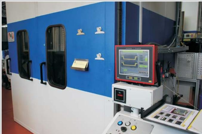
The monitoring terminal is placed right next to the stamping press. The sensor cables plug straight into the terminal. The following signals are measured: stamping forces and binary signals, such as feed, stock progression, and part ejection. The in-die force-acoustic emission sensors are particularly effective, permitting individual forming, piercing, blanking, and bending operations to be monitored.
