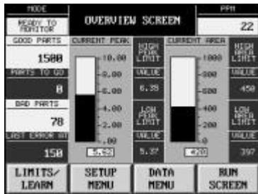
To process the sensor signal, the IMPAX PASS monitoring system was chosen. The PASS monitor observes the power signature of each cycle, and enforces customizable tolerances on the upper and lower bounds. The results of each cycle are displayed on a large graphical screen, along with a trend view to identify changes over time. The monitor tracks the total power signal, as well as the peak power of each cycle, which is often indicative of tool wear (see summary screen at left).
